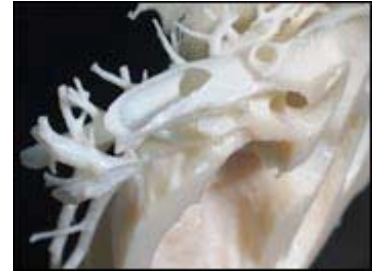
This is a medical model using the additive process called Polyjet. The model was built using a .001" layer thickness using VeroWhite material.
