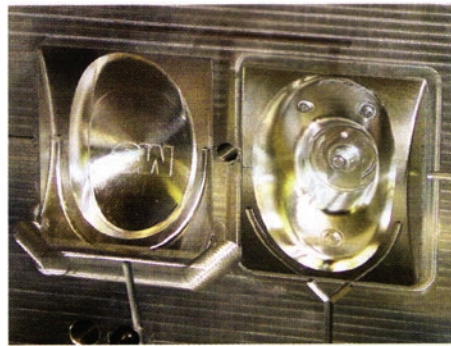
A core and cavity of a 1+1 family tool of the hand sander top handle. The mold finish is as machined.
