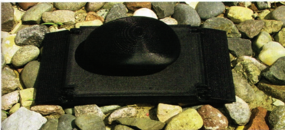
This prototype was made using FDM technology. The part was made from extruded black ABS and was used for some functional testing.
