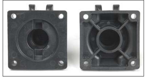
The part on the left had thick sections that made the part warp. The tool was modified to core out the thick areas on the right to produce a quality part.
