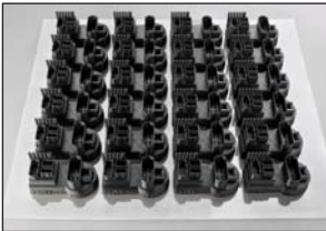
This is a platform of FDM parts used as DDM. The material is black ABS. No tooling was needed to manufacture these parts.
